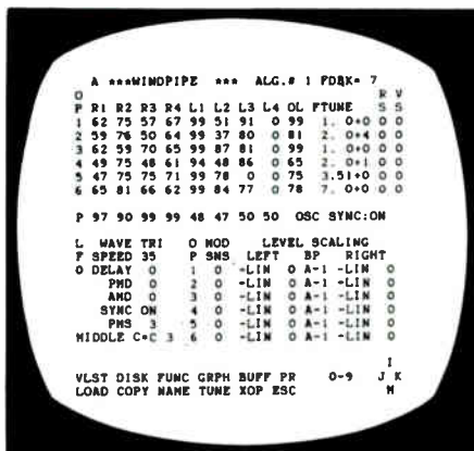
The DX-HEAVEN editing system, from Cherry Lane Technologies, facilitates the creation of voices on the Yamaha DX series synthesizers, as well as provides storage of over 800 voices on a single floppy disk.
