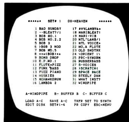
The DX-HEAVEN editing system, from Cherry Lane Technologies, facilitates the creation of voices on the Yamaha DX series synthesizers, as well as provides storage of over 800 voices on a single floppy disk.
