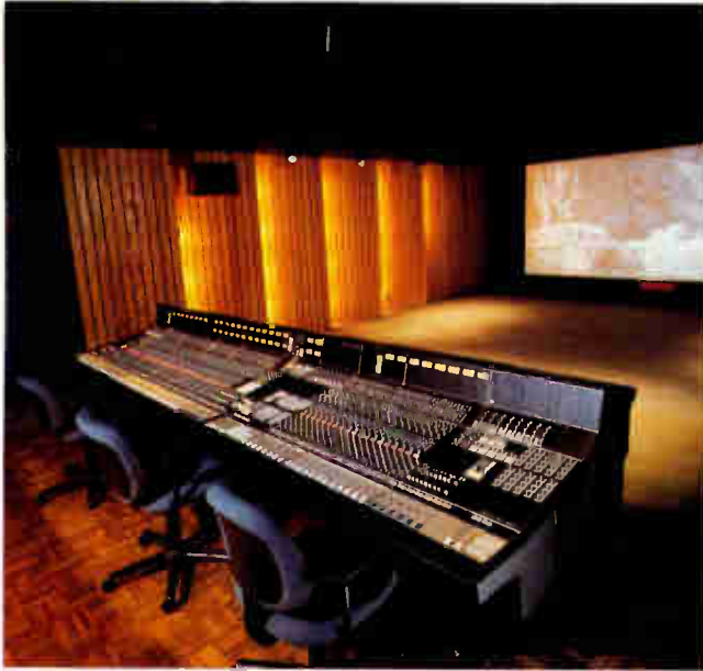
The Stage D film mixing facility at Todd AO Studios East, NYC, features a Solid State Logic 5000 M Series film production system, configured with 60 inputs and a G Series computer with Total Recall and Instant Reset.
