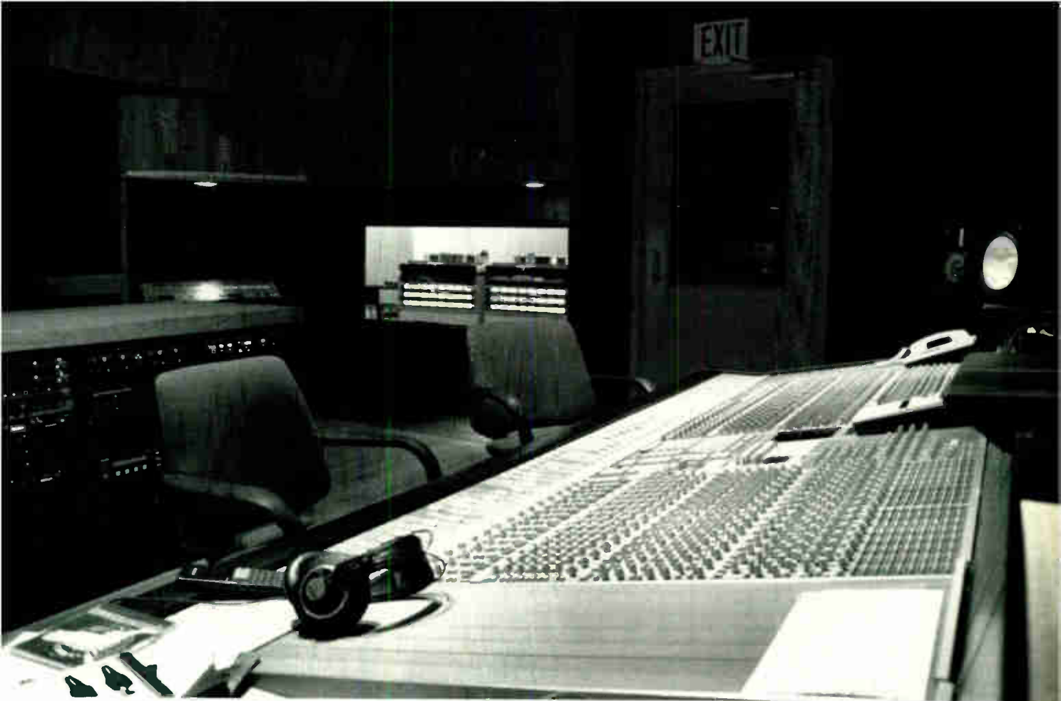
Pictured above: The control room of Vancouver Studios' B room. It features the Solid State Logic 4056 G Series console, with Total Recall, autoscans, patchable VCAs, and 48 mono and eight stereo strips.
