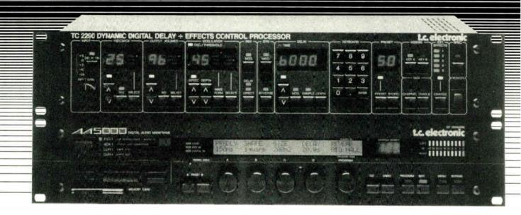
TC 2290: Frequency Response: 20-20KHz, +0 / -0.5 dB THD: < 0.05% 1kHz, 0 dBm; Dynamic Range: >100 dB Digital Conversion: Dynamic Differential Sampling Rate: 1MHz; Max. Input Level: +22dBm
