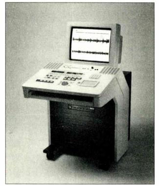
is designed to simulate a modern 2track deck more than a computer system. Also incorporated into the top surface is an "Unmouse," a compact glass tablet controller, which—after a brief period of getting used to—provides fast, accurate system control. Of course, those who prefer traditional mouse control can access the Mac mouse at any time by opening the keyboard drawer.
