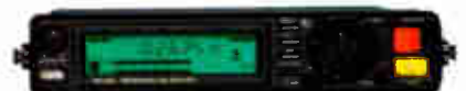
PDR1000 4 head, 4 motor portable professional DAT recorder with 44.1/48/32kHz recording, balanced XLR analogue I/O and AES/EBU + SPDIF digital I/Os.
