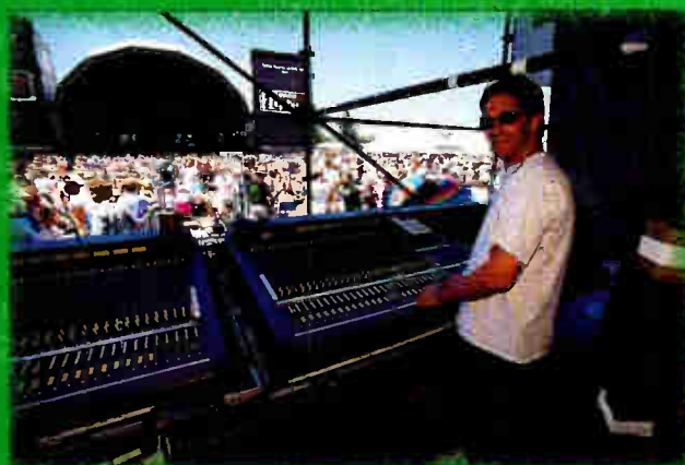
Dan Cleland, The Chieftains' tour manager, usually mixes monitors rather than front of house, but he filled in for engineer Mark Horton who had gone over to another tour. To help The Chieftains stand up to the louder rock 'n' roll bands on the tour, Cleland uses "a lot of specialty mics that help us get gain—a lot of little clip-ons. We use the AKG 419, 409s, 408s, and we really close-mike to get as much gain out of the system as we can. For example, it's very hard to get a lot of gain out of an Irish harp, because the instrument itself doesn't have a lot of volume to it, so we stick on AKG 419 inside the soundboard. It's not the most natural sound sometimes, but we get the vibe, which is what we need for these outdoor gigs."
