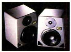
Featuring a 6-1/2-inch polyvinyl proprietary long-stroke woofer and a 1-inch silk-dome tweeter, the crossover point is 1.5 kHz and the sensitivity is 91 dB (1 watt at 1 meter). Maximum SPL is 104
