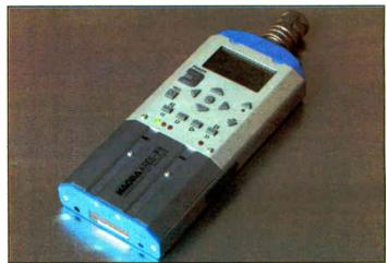
The PC- and Mac-compatible Ares-PII PCM recorder uses a FAT16 file format.
