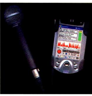
PocketREC loads data onto the DAW or playback system at the studio or docking system, ISDN, mobile phone, modem or direct Internet connection. The transportation of a laptop or tablet computer and recorder to an assignment is rendered unnecessary.
