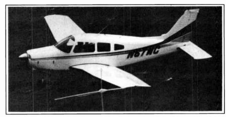
A wing-mounted antenna helped Air System Technologies collect test data from the air.
