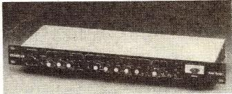
Offering separate compression, expansion-gating, and overall peak limiting, the "COMPEX 2" improves upon Bremerton, WA-based **Audio & Design**'s previous model. With an extension of softer ratios and thresholds to -60dB below normal operating levels, it's possible for stations to process a wide range of dynamics throughout the programming day at a ratio as low as 1.25:1.
