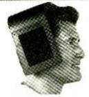
nlike conventional headphones, which bend the wearer's ears out of their natural shape and thus inhibit the normal tonal range of hearing, these "pressureless headphones" developed by Swiss engineer Jurg Jecklin rest lightly on top of the user's head and allow the external ear to guide sound to the eardrum,
