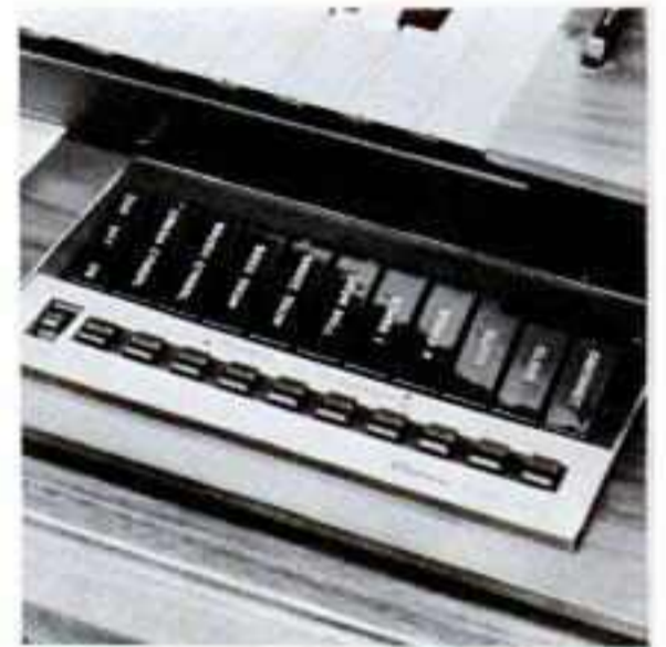
THOMAS ORGAN CO. reports that it sells more than 70 per cent of its organs with built-in Band Box, a versatile rhythm unit designed especially for electronic organs. The unit features 10 voices: crash sycmbal, brush cymbal, bass drum, snare drum, drum roll, bongo I, bongo II, block, clave and castanet.
