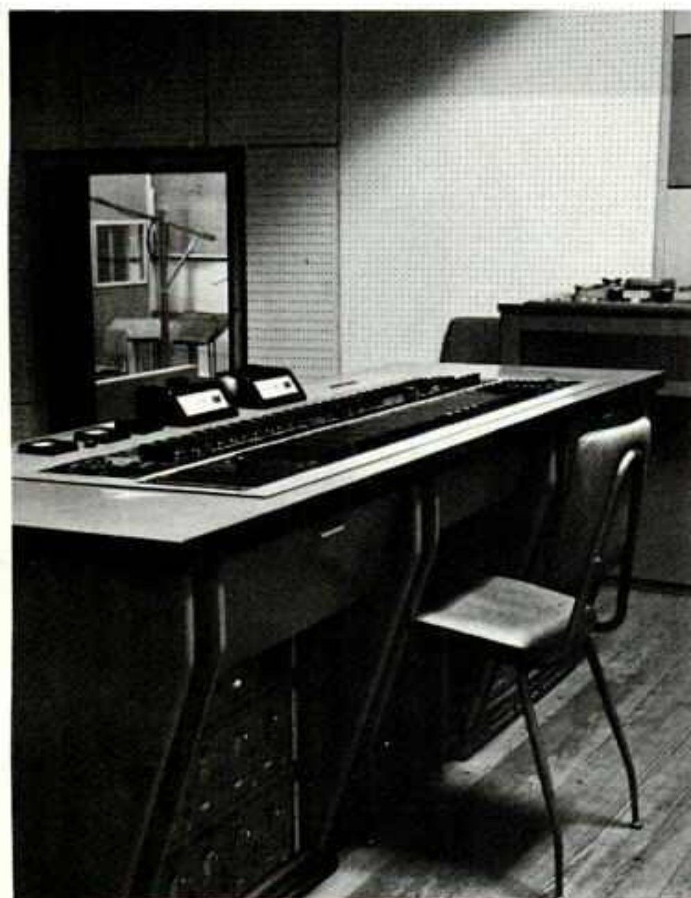
The mixing console in operation at Studio No. 1 which is used for recording on eight-track, one-inch tape.
