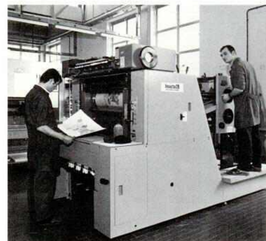
An Invicta 28 four-color rotogravure press turning out top quality graphic reproductions at high speed.
