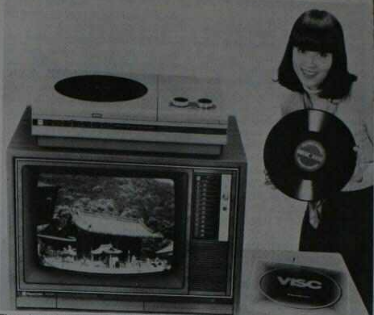
First view of Matsushita VISC player and disk shows machine prototype with simple two-knob operation, standard PVC Panasonic Visc (30 or 60 minutes/side) and experimental package similar to multi-LP "opera box," with molded insert.
