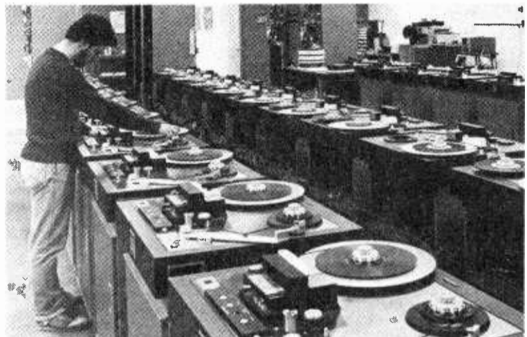
CASSETTE CHECK—An employee of WEA Manufacturing's new plant in Olyphant, Pa. checks one of the many tape duplicating machines.
