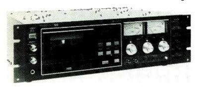
TASCAM RECORDER—This Tascam cassette deck, model 122-B, is designed for use in recording and broadcast studios, and with sound reinforcement systems. It features front panel bias and record level calibration trimmers, and presets for normal, chrome and metal tape. Its three-head design allows simultaneous off-tape monitoring during recording.
