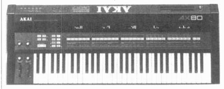
In the VCF section, along with normal filtering operation, the AX80 has EG depth, key follow, key velocity, and a high pass filter.
