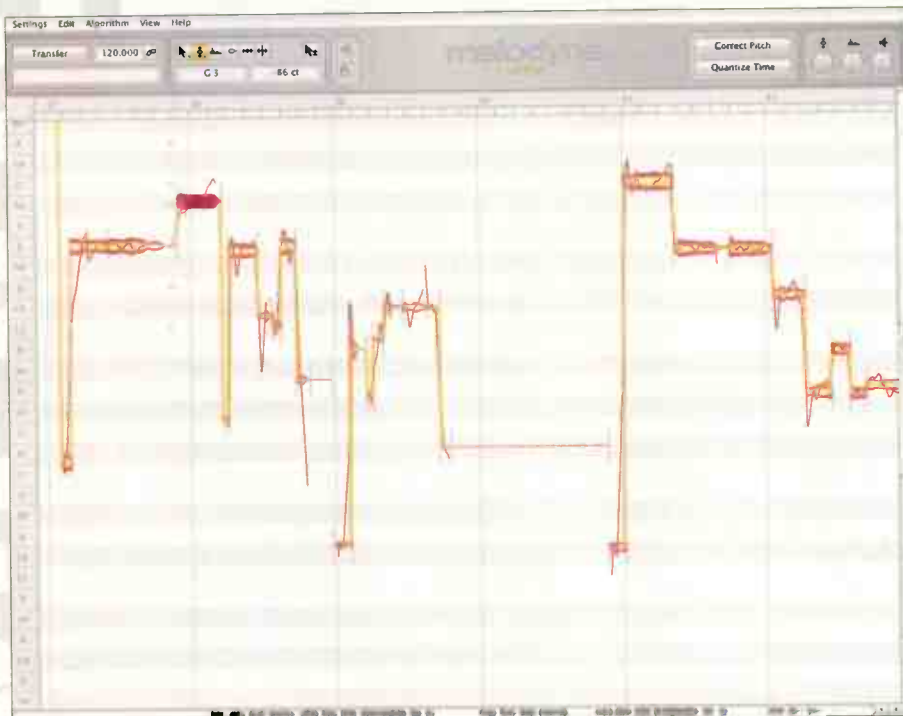
Fig. 1. In Celemony Melodyne Editor's GUI, individual notes of a melody can be dragged up or down graphically to change their pitch.
