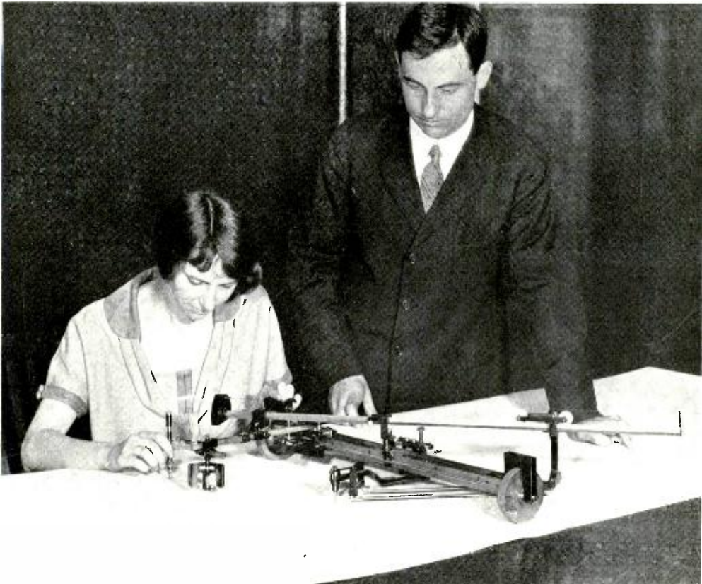
A Scientific Instrument in Action Miss Fessie Smith operates the Coradi Integrator, while Dr. Fry watches the resulting integral curve appear
