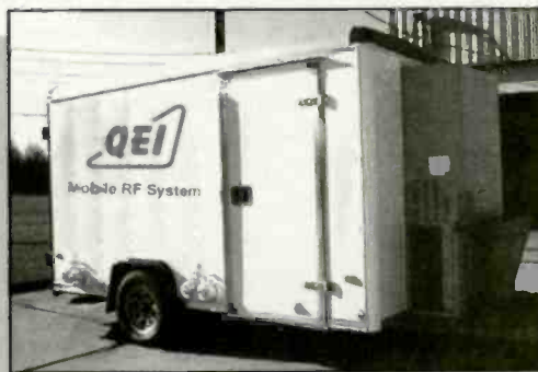
Transportable Pre-Built Transmitter Sites
