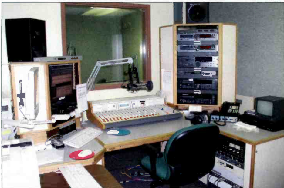
WLRN's Radio Reading Service programming for the visually impaired is transmitted over a 67kHz subcarrier, which is monitored by a Belar RF monitoring system.
