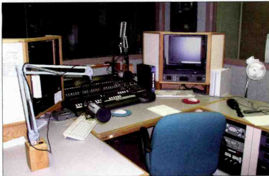
All three production studios will transition to digital in the near future. This studio features a hybrid analog/digital Mackie audio mixer, although the output from the studio remains analog.
