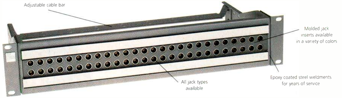
PPV2226RS-SVJ - 2 RU Standard Size 2x26 Super Video Jack Panel
