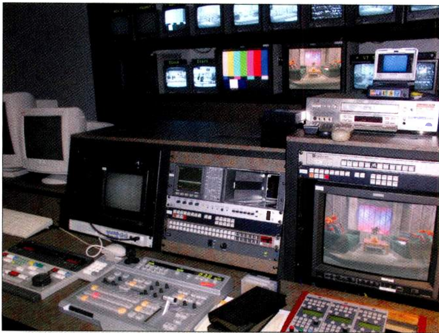
Production control on the lower floor is generally used for KCSB-TV productions but also serves as a backup to the ICTN news operation upstairs. A Ross Synergy One production switcher and an Ikegami monitor are among the visible components in this photo.
