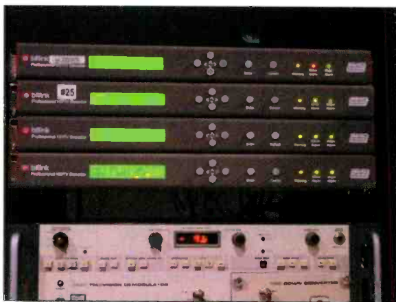
After its transition to digital, KAET-DT selected the BitLink IRD from Digital Vision to perform multiple broadcast functions for the station's main HD program. It will soon use IRDs for SD programs as well.
