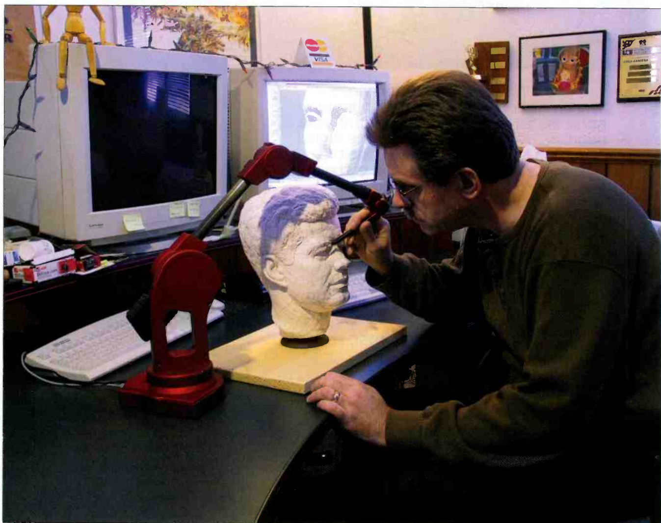
With a digital probe, animator Dale Myers imports data points from a grid on a bust of JFK into his animation system.
