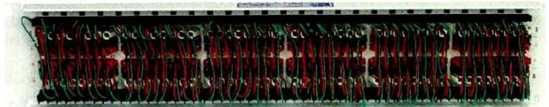
I-96B-MKIV Rear View Showing Jumpers
