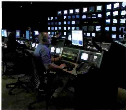
In the KNTV control room, the stations' iNews newsroom computer system drives a Deko MOS interface so CG and graphic insertion can be controlled straight from the desktop.
