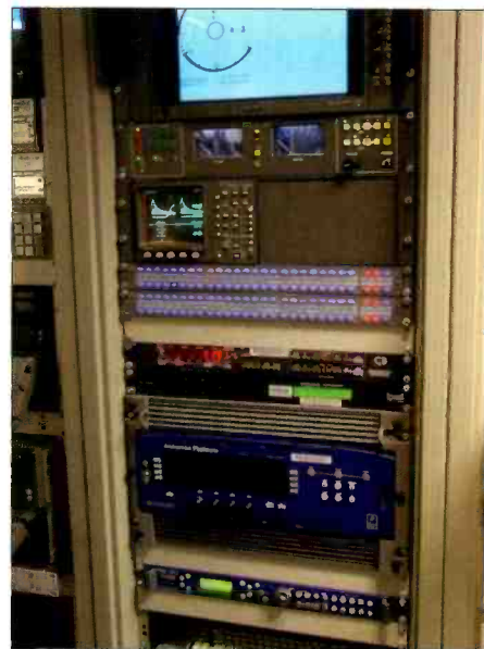
London facility On Sight uses the Alchemist Platinum Ph.C from Snell & Wilcox for upconversion from SD to HD of general material for U.S. and UK consumption.
