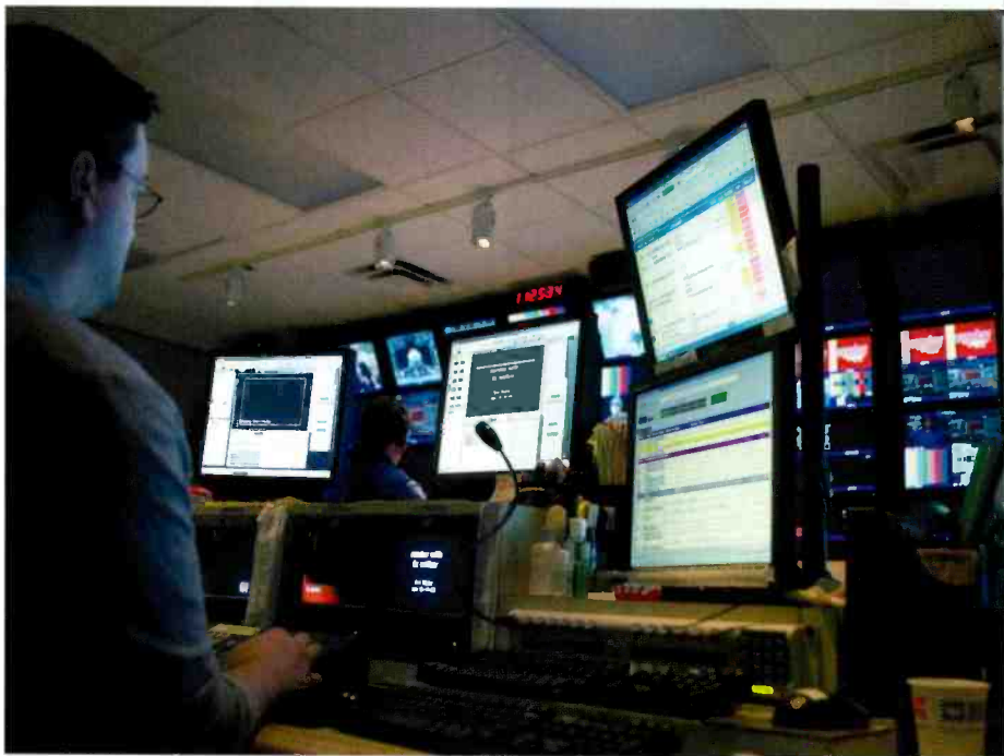
Programming is played to air with automation-assisted playback using iNEWS ControlAir.
