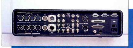
QuBit's rear panel allows a user to hook up to a variety of broadcast equipment, as well as to computer workstations.
