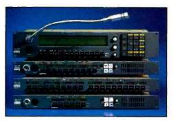
From the top, a 12-key LCD display station, a 9-key LED display station, a 20-key LED expansion panel, and a 5-key LED display station.
