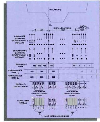
Figure 1. Structure of 4:2:2 digital sampling as per SMPTE 125M. (For more information, see "Transition to Digital," August 1995.)
