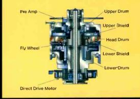
To ensure S-VHS compatibility, the drum structure features an upper stationary drum, a middle rotary drum, and a lower stationary drum. To eliminate the need for a thicker air film at the drum inlet and to provide stable head-to-rape contact, the thickness of the rotary drum is very narrow. The end result of this configuration is the truest track linearity. The inner drum's tapered shape also reduces tape damage, powder drop, wear and burn.
