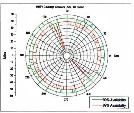
*Figure 5.* Antenna contours that would result when the installation of Figure 3 is combined with the power penalty of Figure 4.
