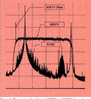
Figure 1. The spectra of undistorted NTSC and HDTV channels.
