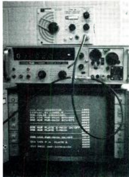
Figure 18. Video test generator (Tektronix 191) with frequency counter
