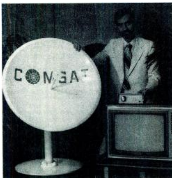
The Comsat direct-to-home terminal might consist of a small dish and decoder like those pictured
