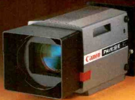
PV14x12.5BIE High Resolution Lens for 30mm and 25mm cameras. A Unique Design —featuring extensive use of Fluorite lens elements, this lightweight, compact 14X studio lens provides high sensitivity and critical sharpness at all focal lengths. Focal length: 12.5-175mm (1.5X and 2X extenders built-in) Max. Relative Aperture*: 1:1.6 at all focal lengths *25mm format
