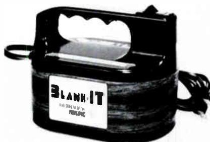
able of erasing magnetic tape of all formats, including audiotape of up to 1 inch, computer tape, and both VHS and Beta videocassettes. Thermocouple protected, the unit shuts off when its duty cycle has been exceeded. After a short cooling period, it is operable again. Duty cycle for the unit is five minutes on, 15 minutes off.
