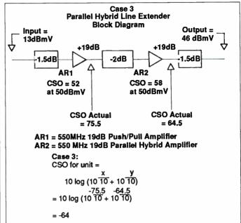
ing amplifier and line extenders will both be parallel hybrid units, meaning that the push/pull hybrid will be used as the input with the parallel hybrid device used as the output. Levels for the units will be +11 dBmV input; 37 dBmV output for the trunk; and the
