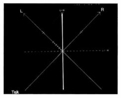
Figure 2: Left and right channels matched in phase and gain.
