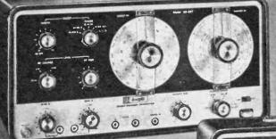
B RF Generator with Built-In Crystal Calibrator
