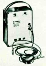
The transmitter sends out a signal when pushbutton on dashboard is pressed. Re-ceiver in the garage picks up the signal, turns on the overhead light and starts the motor to operate the lifting mechanism. The next time the button is pressed, the motor will reverse to close the door and lock it securely. Crystal-controlled opera-tion on FCC-authorized frequency of 27.255
