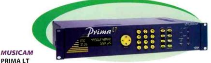
The bi-directional stereo Prima LT ISDN codec comes with Musicam-enhanced MPEG Layer II, MPEG Layer III and G.722 algorithms for maximum compatibility. It accepts one digital interface module for direct connection to ISDN, V.35, X.21 or RS422. Features: 24-bit A/D and D/A converters; dynamic range better than 92 dB, ultralow distortion at less than 0.01%; data rates to 384 kbps; built-in terminal adaptor for U.S.; optional AES/EBU and S/PDIF I/O.
