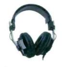
The Fostex T20RP headphones can handle high SPL without distortion. They offer sturdy construction with soft, comfortable fit in a semi-closed format. Removable cable is easily replaced. Frequency response 50 Hz to 30,000 Hz. 1/4" TRS connector.
