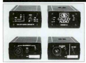
A test instrument, for the audlo installer or soundman, which Indicates absolute polarity of most audio devices or may be used as a cable tester. The send unit has balanced 1/4" and XLR jacks, an unbalanced 1/4' speaker out jack and an internal speaker. The receive unit has 1/4" and XLR jacks, a sensitivity control, and an internal mictophone. Both units are housed in high Impact padded ABS case and are powered by a 9 volt battery
