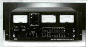
The TFT 844A is an FM stereo mod monitor that has a frequency aglle RF pre-selector, baseband demodulator and stereo demodulator. The 844A can be used for off-air monitoring or direct transmitter proof measurements. This monitor can be used for complete measurements of total, right and left channel modulation, channel separation, main
