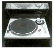
The Technics SL-1200MK2 is a quartz-locked direct drive turntable that is virtually feedback-proof because of its special base design. The platter is damped on both sides to avoid ringing. Its high starting torque brings the platter to rated speed within 0.7 second. Includes base, tonearm and dust cover. 331/3 and 45 RPM  $\pm$  8% pitch control.
