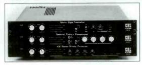
The CRL SGC-800 is a stereo AGC/compressor which is used before an STL or telco lines to eliminate system overloading. The AGC can be operated as "dual-band, wideband or both" and allows for up to 30 db of galn reduction. Dynafex® noise reduction is also included.
