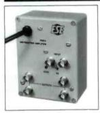
The ESE 207 and 208 compact video distribution amplifiers are portable and easy to install. Controls are easily accessible for video galn, DC level and HF equalization. The amplifiers are clamped to provide a consistently stable output signal to the output terminals. A single pair of BNC connectors are wired for a loop-thru input with provisions for a terminating resistor if desired.
