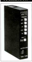
Battery operated 5-frequency sine wave oscillator (40 Hz, 400 Hz, 1, 10 and 15 kHz) with 3 selectable output levels (-30, -10 and O dB) Is useful for spot checking frequency response, calibrating mixers with tape recorders and other level matching Jobs.
