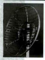
Mark Antennas meet or exceed every existing F.C.C. requirement, are lightweight, strong, heli-arc welded aluminum, multielement parabolic grid antennas. One of the outstanding characteristics of a grid antenna is the low wind loading figures, usually 25 to 40% of solid dishes. When ordering please specify frequency.
