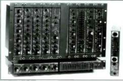
The Rane Flex modular signal processing series offers a wide variety of high performance audio procession, mixing, and distribution modules.
