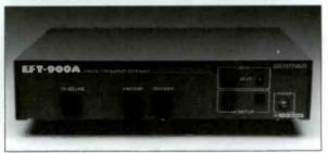
Gentner's EFT-900A is self-contained to keep equipment needs low at remote sites. It has a built-in telephone coupler, mlc preamp and headset amp. The EFT-900A provides two-way operation and is ideal for sports or sales remotes.
