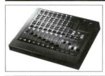
The Sony MXP-290 audio mixer features 8-channel operation with 48V phantom power, 3-band equalization, and +4dB balanced line input. An internal preview switcher is controllable from Sony editors via parallel mixer interface.
