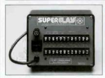
The Henry Superelay is a quick and easy relay Interface for use in any studio installation requiring multiple circuit control. Superelay provides six double-throw relay outputs for low-voltage and audio switching. It can be controlled by any switch, momentary or maintained relay, or CMOS/ TTL logic circuit. The AC output is switched with a solld-state synchronous relay for direct powering of "On Air" warning lights. Includes an internal flasher circuit and 12 VDC/250 mA utility power supply.
