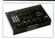
The Telfax GX-440 has all the features of the GX-400 plus a second phone line that allows the announcer to alr calls from listeners while at the remote site. This second line can also be fed to the announcers headset to listen for cues from the studlo while broadcast-
