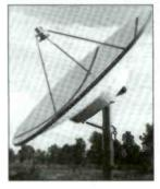
Comtech's 3.0 and 3.8 meter antennas keep installation costs down with a single pole mount and three-piece reflector design. The use of Comtech's unique splice-strap system yields a superior surface tolerance. The 3.8 meter has a gain of 42.9dB, ideal for SMATV, radio SCPC and Cable TV applications. The El/Az mount permits 360° azimuth adjustment without costly foundation alignment. The elevation jack provides smooth elevation adjustment from O to 70°. The polar-mounted system
