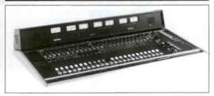
The 800 series console is available in 12, 18 and 24 maInframes. It is available with: stereo program, audition, utility and auxilliary output busses, 2 mono mix-minus output busses, L+R output summlng, and 2 line telco module. This console has an extensive user-programmable logic control system. All push button controls are electronic with LED status indicators. All faders are stereo-balanced controlling VCA's.
