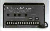
Henry's Micromixer will accept up to four balanced or unbalanced line-level inputs and will mix them to a stereo output. A level control for each input provides adjustment from "off" to + 10dB of gain. "Micro-Assign" switching permits each input to be assigned to the left, right, or both outputs in any combination. All circultry is active and direct coupled for exceptional sonic accuracy.
