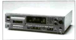
The Sony PCM-2300 professional digital audio tape recorder /player has balanced analog and coaxial digital IEC-958 Ins and outs, long play mode, auto fader, margin display, records absolute time, supports three sampling frequencies, and is supplied with a wired/wireless remote and rack mount adapters. In the long play mode it can hold up to four hours of 12 bit non-linear 32kHz audio.
