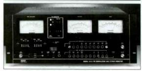
The TFT 884 is a cost effective alternative to the 844A. All proof measurements can be made along with incidental and residual synchronous and asynchronous AM noise. It includes a convenient front panel test output. The 884 has a one year manufacturer's warranty.
