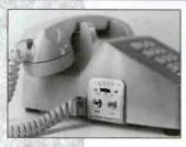
R/SVP is an audio coupler built in the standard U.S. made 2500 series touchtone phone. The panel on the phone base has an 8  $\Omega$  send jack for direct connection to cassette recorders or other electronic sources and a low impedance record jack to provide a clear balanced signal to record conversations. The amplified electret condenser microphone has superior voice quality. R/SVP comes complete with telephone and modular plug line cord.
