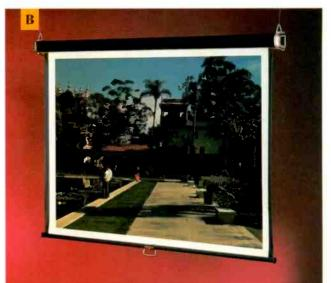
To Calculate the Screen Size: Determine the distance between the screen and the last row of the audience. Divide that distance by 6 for screen width of 4x3 ratio projected images, or divide the distance by 8 for screen width of square projected imagest Matte White is an excellent general purpose surface, the best choice for most requirements in Education and Training. Light is reflected almost equally in all directions, and the brightness level is constant from any viewing position,
