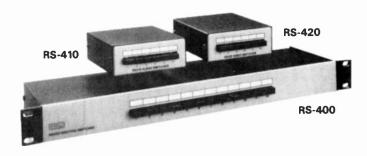
The switchers contain no active electronics and consume no power. High quality switches with gold contacts are used for high reliability operation. Gold plating is also used on all the audio input and output connectors to improve reliability. All unselected inputs are internally terminated to help minimize crosstalk. All pushbuttons are interlocking.
