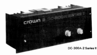
monic and intermodulation distortion with very low noise. A switch on the rear of the unit allows stereo or mono operation with no internal wiring changes. In the mono mode, the DC-300A-2 is capable of a 70V balanced line output. The unit operates on AC current from 120V to 240V. 155W continuous average power per channel into 8 ohms at .05% THD.
