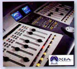
That's right...Ethernet. A 100Base-T segment, using a standard C AT-6 cable, can carry 25 stereo charmels of 48 kHz, 24 bit linear PCM audio in both directions; a 1000Base-T link or Gigabit fiber can carry hundreds of channels. Segments are connected using modern Ethernet switches to enable a single network to carry in excess of 32,000 stereo channels! All for about half the cost of a traditional hardwired routing switcher.
