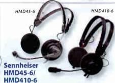
The Sennheiser HMD45-6 and HMD410-6 headsets offers lightweight and comfortable construction, with open, split headbands and quality dynamic supercardioid mics. Each offers a slightly different headband design. Headphone frequency response for both is 20 Hz-18 kHz; impedance is 600 ohms. The HMD45-6 microphone frequency response is 100 Hz-12 kHz; impedance is 200 ohms. The HMD410-6 microphone frequency response is 50 Hz to 12 kHz. Cables are unterminated.
