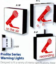
Prolite Architectural series lights are attractive and functional. The housing and canopy are triple ground, cast aluminum with a baked, matte black enamel finish. Dimensions are 7.5" square with .75" high letters with large microphone image. Two 20-watt, 6.5" longlife lamps are supplied. Choose from three different configurations: single lens flat wall mount, double lens wall or ceiling mount, or double fens ceiling pendant mount. Extra lenses also available.
