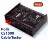
The Rolls CS1000 tests ten cable types including banana, balanced/unbalanced 1/4" and 1/8", RCA, Neutrik Speakon, XLR female, XLR male, MIDI (7 or 5 pin DIN), RJ11 (telephore), and RJ45 (Ethernet and CAT-5), with LED indicators. In addition, the CS1000 features a 1 kHz test tone oscillator and phecks phantom power voltage and polarity (signals present).
