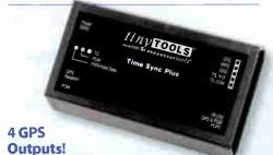
The Time Sync Plus provides four GPS time referenced outputs. The first is an SPST relay, which pulses at 12:00, 22:00, 42:00, and 54:30 and is userprogrammable in each of four locations for any minute and second. The second is an active high driver with a 100 ms pulse each second, while the third is a 4800-baud, RS-232 serial port providing a time zone adjustable time code. The forth provides an active high driver in the ESE TC-90 serial time code format.
