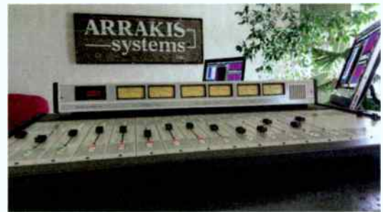
MARC Series 15 Channel - 3 Stereo Output Buses Modular analog, up to 30 (A/B) inputs.
