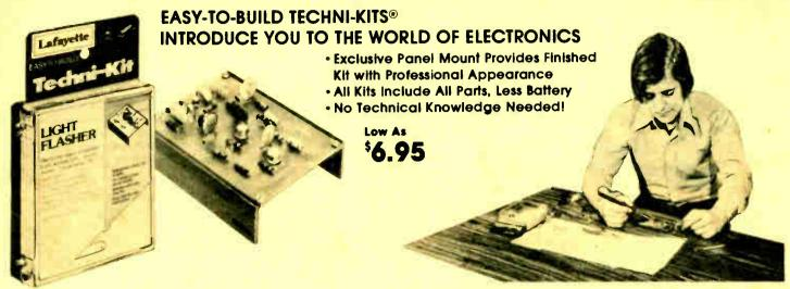
TK-1000 Light Flasher Kit. A 2-transistor "flip-flop" batteryoperated multivibrator circuit alternately lighting two bulbs. Ideal for use in displays, signaling and warning devices. Educationally demonstrates the basic fundamentals of the widely used multivibrator. Uses 6-volt battery (order below). 19 P 01255V Wt. 8 oz. ......\$6.95 32 P 48184 6V Battery 1 lb. 12 oz. 1.65
