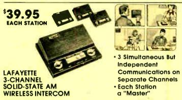
Features call button with pleasant tone, press-to-talk bar with "lock-talk" button for continuous monitoring plus volume and channel selector. Advanced circuit design with built-in pre-set squelch and AGC to prevent overloading and provide high isotation between channels. Dependable fused transformer power supply with pilot light. Solid state circuitry with 5 transistors, 4 diodes. Size: 7½W x 5½D x 2¾'H. For 117 VAC, 60 Hz. Imported.
