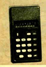
This efficient little calculator adds, subtracts, divides and multiplies. Has floating decimal which positions decimal point in answers automatically. Features minus sign, overflow indicators, easy-to-read red digital display. 4½ x 2½ x 1".
