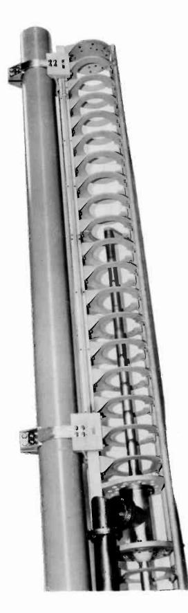
A Portion of a Type 1046-R Antenna Bay Mounted on its Supporting Mast
