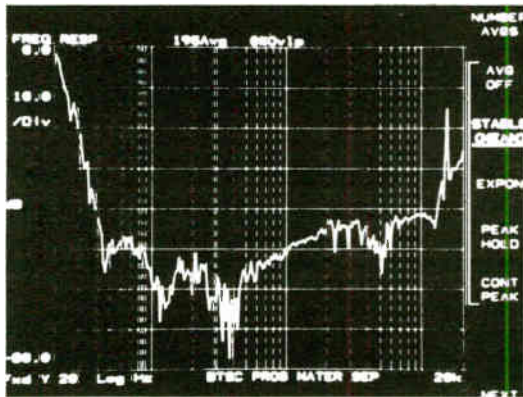
Fig. 4: Separation Performance (Measured with dual-channel FFT, using program material)
