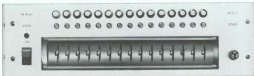
The Programmer sequences the program sources in the system.
