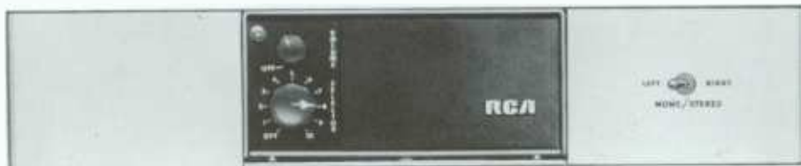
Automatic Cue System allows off-line use of program sources.
