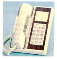
Radio Shack ET-192. Auto-dials up to 20 numbers of up to 16 digits each. Programmable Touch-Tone or pulse dialing lets you use computerized services from a rotary line. Flash button for use with services like Call Waiting. Touch-redial, ringer-adjust, comfortable "K"-style handset. Removable woodgrain lets you customize laceplate with your own fabric or wallpaper. With CR 2032 memory backup battery. 43-532 . . . . . . 49.95
