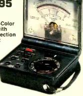
Fuse/surge-absorber protected. Sensitivity: 20,000 ohms per volt DC. Measures to 1200 volts DC in seven ranges, 1200 volts AC in five ranges, DC current to 300 mA in four ranges. Resistance to two megohms; dB: -20 to +63 in five ranges. Accuracy ±3% DC, ±4% AC. Open 71/4 x 45/16 x 11/4". Requires "AA" battery.
