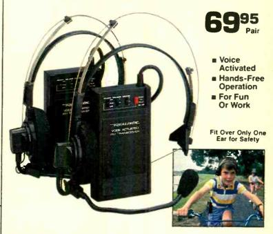
Realistic® TRC-500. Voice-activation leaves your hands free while you talk with a companion. Sensitivity switch lets you adjust the level of voice activation—you can prevent unwanted transmissions during strenuous activity or pick up soft voices when necessary. Volume control. 49 MHz FM dual-conversion receivers with 1/2-microvolt sensitivity. Up to 1/4-mile range. Switchable VOX/manual operation. With belt clips. Each headset requires 9V battery.
