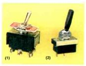
(1) Heavy-Duty DPDT With Center Off Position. Rated 10 amps at 125 VAC. Features screwdriver terminals for easy hookup and includes on-off-on label plate. Body size: 3/4 x 13/8 x 13/8". Mounts in 7/16"-diameter hole. 275-1533 . . 1.79
