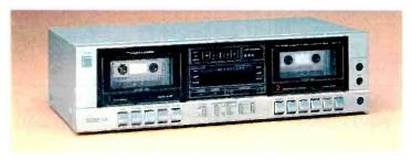
Response  $\pm 3$  dB: 60-14,000 Hz (metal). 60-12,500 Hz (CrO\_/Hi-Bias). 60-10,000 Hz (normal). Wow and Flutter: 0.12% WRMS. S/N: 60 dB Dolby (ref. 3.0% distortion, "A" weighted, metal tape). Distortion: 1.0% 3rd HD. Record/Play Head: Permalloy. Erase Head: Ferrite. Size:  $49_{16} \times 169_{16} \times 8^{1}/4"$
