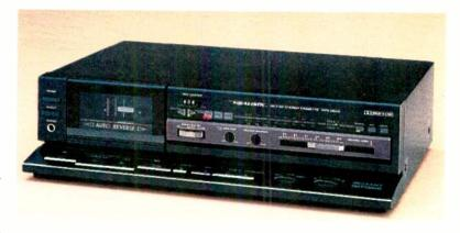
Response ± 3 dB: 40-16,000 Hz (metal), 40-15,000 Hz (CrO<sub>2</sub>/Hi-Bias), 40-14,000 Hz (normal). Wow and Flutter: 0.06% WRMS. S/N: 70 dB Dolby C; 62 dB Dolby B (ref. 3.0% distortion, "A" weighted, metal tape). Distortion: 1.5% 3rd HD. Record/Play Head: Permalloy. Erase Head: Ferrite. Size: 43% x 17 x 83%."
