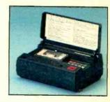
Can be triggered by an alarm system or by the touch of a button. Dials up to three numbers in sequence and plays your prerecorded message. Monitor switch, built-in mike, message-is-playing and battery-check LEDs. Battery-backup system in case AC power fails. Works on any pulse or tone line. UL listed AC. Backup requires 3 "AA" and 4 "C" batteries. FCC registered 31/2 × 9 × 61/2" 49-431 99.95
