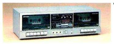
Response ±3 dB: 40-14,000 Hz (metal), 40-13,000 Hz (CrO<sub>2</sub>/Hi-Bias), 40-12,500 Hz (normal). Wow and Flutter: 0.15% WRMS. S/N: 60 dB Dolby B: 50 dB (ref. 3.0% distortion, "A" weighted, metal tape). Distortion: 1.2% 3rd HD. Record/Play Head: Permalloy. Erase Head: Ferrite. Size: 5 x 16½ x 8"
