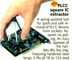
PLCCs and has ESD handles for safe use on static-sensitive chips. 276-2101 .... 9 99
