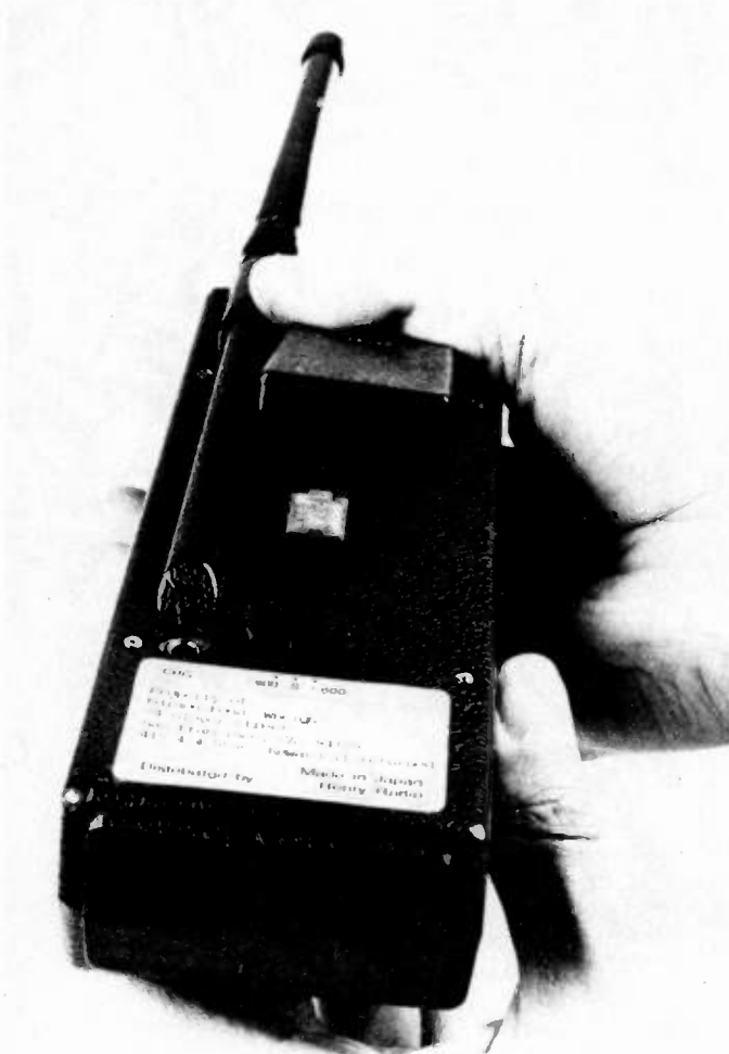
Fig. 8. The back of the transceiver showing the placement of the DIP switch.
