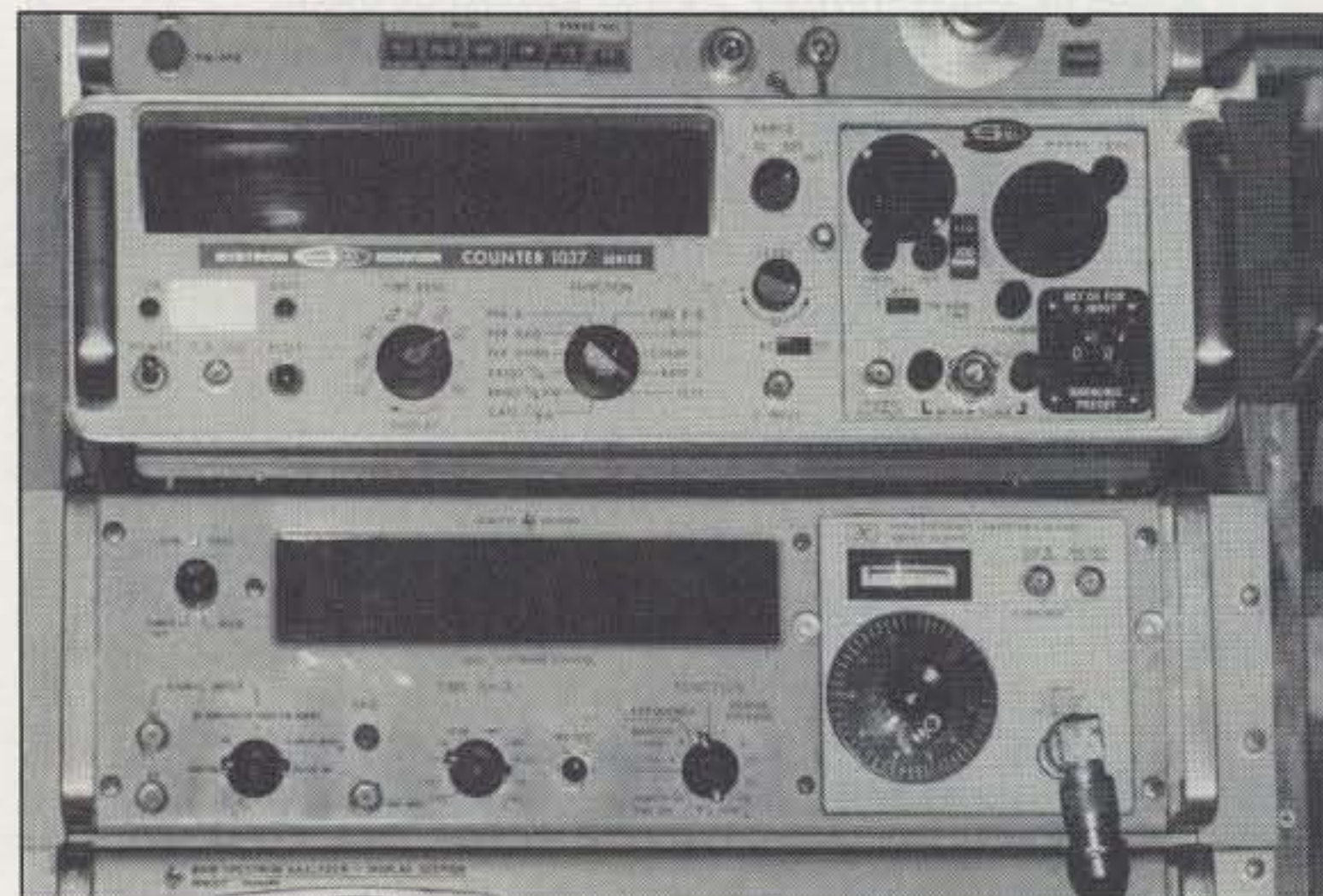
Photo C. Comparison between an HP-5245 with a 3-to-12.4-GHz plug-in (bottom) and a Systron Downer 1037 frequency counter with a transfer oscillator plug-in good to 18 GHz (top).
