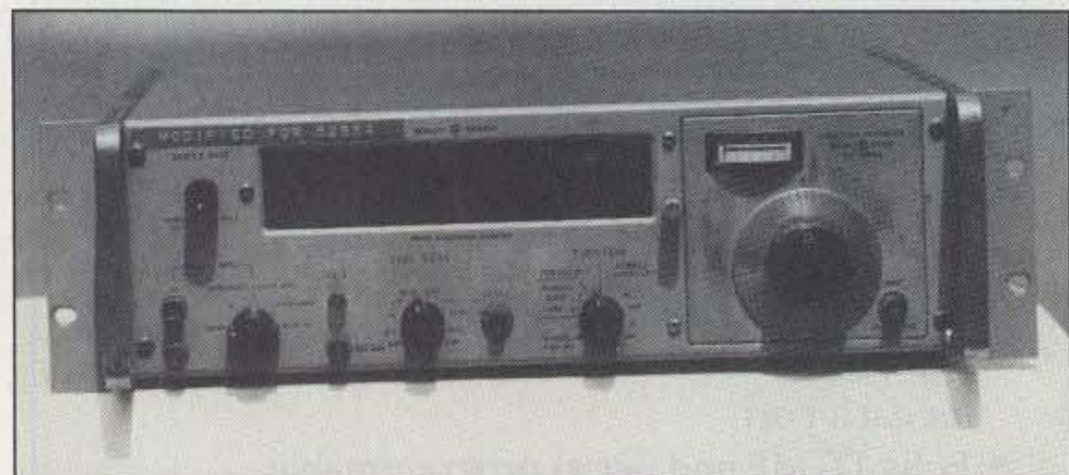
Photo B. My old trusty HP-5245 counter with a 500 MHz plug-in displays 10 MHz frequency to eight digits.
