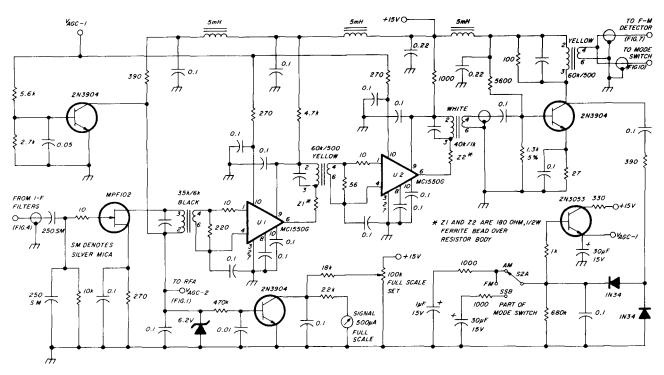
fig. 5. I-f amplifiers and agc detector and amplifier.
