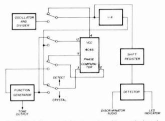
fig. 8. Block diagram of detector and tunable encoder based on encoder-decoder shown in fig. 7.
