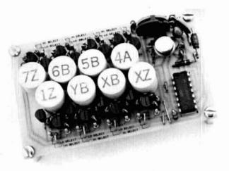
Eight-frequency encoder with ceramic resonators.
