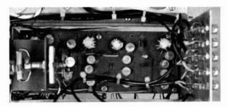
Top view of the receiver showing the rf amplifier and first mixer.
