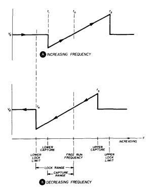
fig. 4. Frequency-to-voltage transfer characteristics of a phase-locked loop for increasing input frequency, A, and decreasing input frequency, B.
