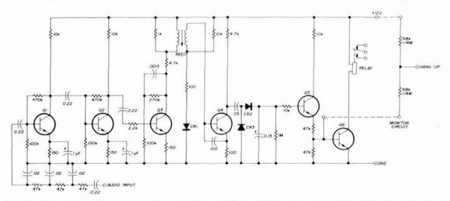
fig. 6. Reed decoder. Transistors are general-purpose silicon npn. CR1 and CR2 are silicon signal diodes. With the monitor circuit connected, the receiver will respond to a signal without *PL* when the "hang up" terminal is ungrounded.
