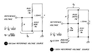
fig. 3. Reference voltage sources for use with the voltage calibrator. In each circuit, R is selected so that it, in parallel with R102, will satisfy the equations shown next to each circuit, within  $\pm 0.2$  per cent.  $R_m$  in circuit B is the input resistance of the DVM. Refer to the text for suitable battery types.
