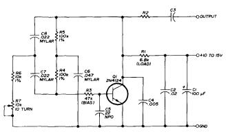
fig. 3. Twin-T oscillator. C1 is not required in battery-powered portables. Select R2 to give desired modulation level.
