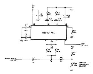
fig. 11. 10.7-MHz fm modulator using the NE560 PLL. Resistor R8 provides  $\pm$  10% variation of the center frequency. For best waveform linearity resistors R4 and R5 should be equal; minimum value for R4 and R5 is 20k.
