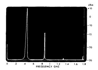
tudes are "stretched" somewhat, as seen in the scope photograph. However, it is possible to measure signal amplitudes to within one or two dB over the entire 40 dB range, once you get the hang of it. It is possible to view spectral components as far down as -40 dBm, but scale compression at the low end is so great that you can only guess at the actual amplitude.
