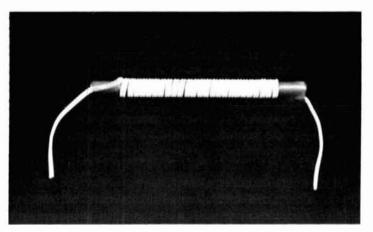
Loudspeaker lead can be wound into an rf choke by winding the lead around a ferrite antenna rod.
