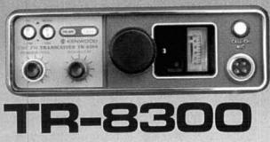
FM transceiver for 70-cm Amateur band. 23 crystalcontrolled channels (three supplied). Transmitter output is 10 watts.
