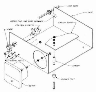
fig. 4. Mechanical details of the enclosure.
