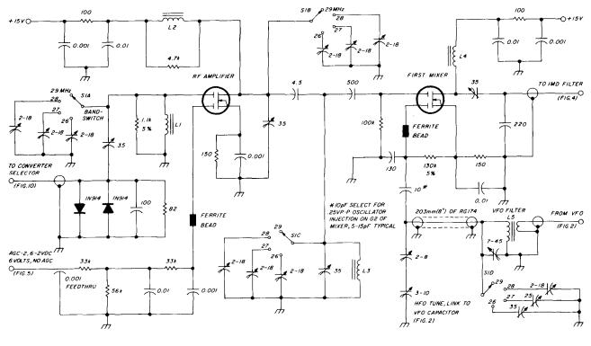
L1 - L5 wound on 13 mm (0.5 in.) OD type E toroid cores
