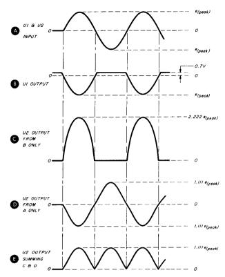
fig. 2. Waveforms of the precision full-wave rectifier circuit.
