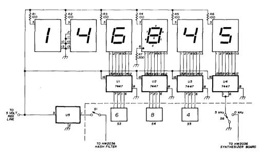
fig. 1. Schematic diagram of the addition to the HW2036 to add an outboard frequency display. Instead of using 7 resistors for each LED, a common current-limiting resistor is inserted in the anode line. The LEDs must be of the common-anode type. The 5-volt regulator is a 7805.
