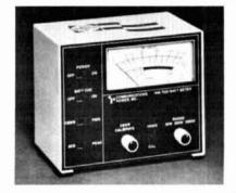
accurate swr readings to a ratio of 1.1:1. Most other swr bridges use 10 dB directional couplers, accurately reading to only 2.0:1, and even some of the more expensive meters only use 20 dB direction couplers.
