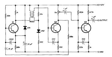
fig. 1. Communications Specialists miniature reed encoder. CR1 and CR2 are silicon diodes. Q1, Q2, and Q3 are generalpurpose npn silicon transistors.
