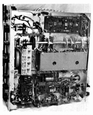
The right-angle gear drive is used to select an i-f filter mounted on the top of the chassis. The four trimmers, behind the dial assembly, are used in the main receiver vfo to select the different frequency segments.
