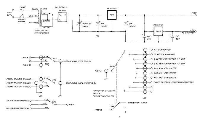
fig. 10. Power supply and switching arrangements.
