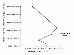
fig. 7. Inversion sounding trace showing temperature changes as a function of altitude between 400 and 2500 meters (1312 and 8200 feet).
