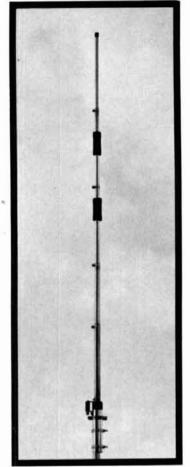
ATV-3 Cushcraft's ATV-3 multiband vertical provides low VSWR operation for both SSB and CW on 10, 15, and 20 meters. Matched to 50 ohms, built-in connector mates with standard PL-259 Stainless-steel hardware is used for all electrical connections. The ATV-3 is a compact 166 inches (4.2 meters) tall. Rated at 2000 watts PEP
