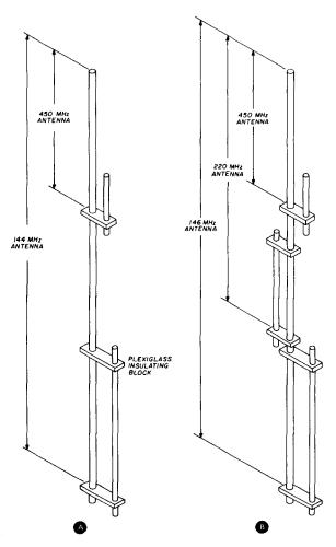
fig. 2. Multiband J antennas for 146 and 450 MHz, A, and for 146, 223, and 450 MHz, B. Antennas built by the author were fed with separate coaxial feedlines and baluns.
