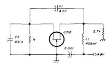
fig. 7. The same oscillator shown in fig. 6, except designed with the more accurate method.
