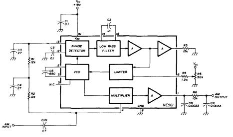
fig. 10. A-m detector for 455-kHz i-f using the NE561 PLL.
