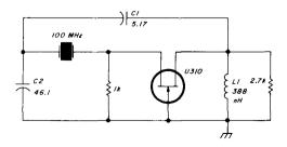
fig. 8. A 100-MHz crystal oscillator which was designed using the same methods as the Colpitts oscillators.
