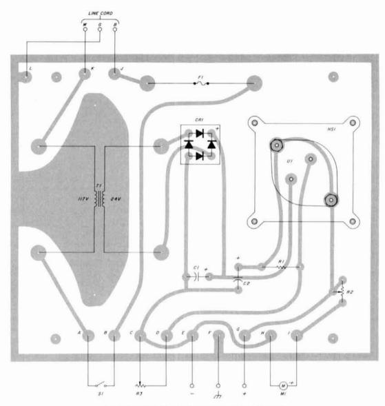
fig. 3. Parts placement diagram for the circuit board.
