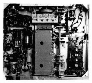
Bottom view of the author's receiver. The two boards in the bottom right are the i-f amplifier and the agc detector/amplifier. In the upper left is the bfo/product detector board. Mounted on the left side of the main chassis are the a-m detector and squelch boards. Below and to the right of the product detector is the audio amplifier board. To the left of the audio board is the fm limiter and detector.
