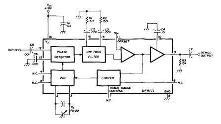
fig. 7. 10.7-MHz fm demodulator using an NE560 PLL IC. Design details are given in the text.
