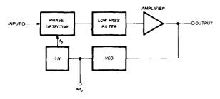
fig. 5. Phase-locked loop frequency synthesizer using a digital frequency divider.
