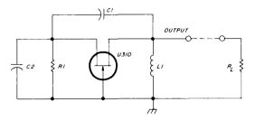
fig. 3. To further simplify analysis of the oscillator, this diagram shows the circuit redrawn into the general form of a common-gate amplifier.
