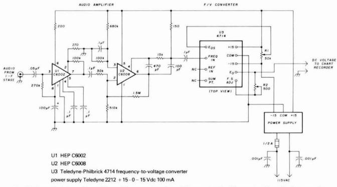
fig. 4. Schematic of the audio amplifier and frequency-to-voltage (FV) converter. The FV converter drives the chart recorder.
