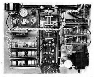
Overall top view of the receiver. The i-f filters are mounted in the upper left. The ICs for the counter are mounted in the upper right. Note the shielding on both sides of the counter board.
