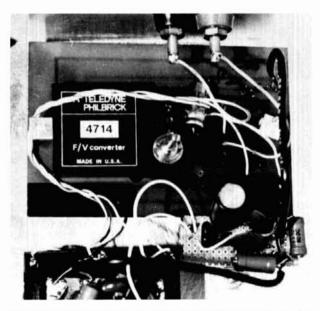
View showing the inside of the audio-processing stage and the frequency/voltage converter.
