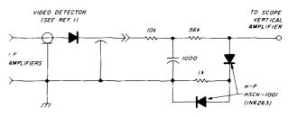
fig. 2. Signal-processor circuit as modified by N6TX for use with his microwave spectrum analyzer.<sup>1</sup>
