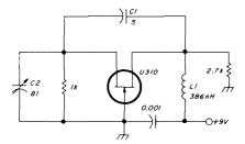
fig. 6. A common-gate oscillator designed with the generalized design technique.
