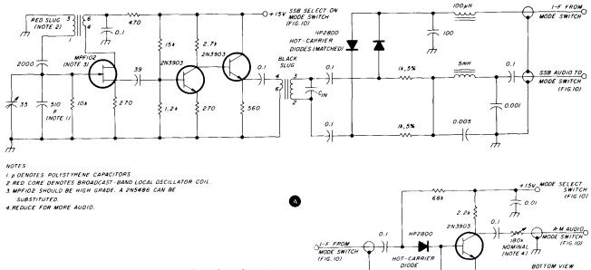
fig. 6. Ssb beat-frequency oscillator and product detector, A, and a-m detector, B.
