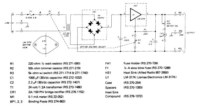
fig. 1. Schematic of the variable-voltage power supply. The lettered terminals are used to indicate where the leads enter and leave the printed-circuit board. All resistors are 1/2 watt tolerance; capacitors are rated at 35 volts dc. RS part numbers are available from Radio Shack.
