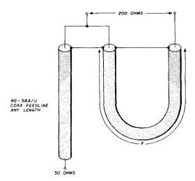
fig. 4. Construction of the half-wavelength coaxial balun. Length F is given in table 1.
