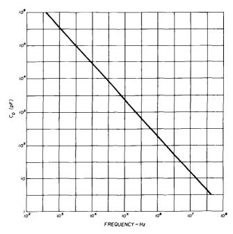
fig. 8. Free-running oscillator frequency as a function of vco timing capacitance.
