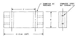
fig. 3. Layout of the aluminum shorting bars and plexiglass spacers. Dimensions C and E are given in table 1.
