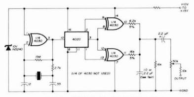
fig. 4. Lake Erie ARA crystal-controlled encoder.
