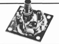
SAX-1 TRANSISTOR RF AMP A small signal amplifier to drive the MXX-1 Mixer. Single tuned input and link output. 3 to 20 MHz, Lo Kit, Cat. No. 035102. 20 to 170 MHz, Hi Kit, Cat. No. 035103. Specify when ordering.
