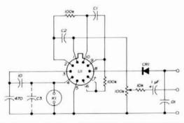
fig. 5. Communications Specialists micro-miniature encoder. Values of C1, C2, and C3 and connection to pin 6 or 7 of U1 depend on frequency. U1 is a custom-made IC; K1 is a ceramic resonator.
