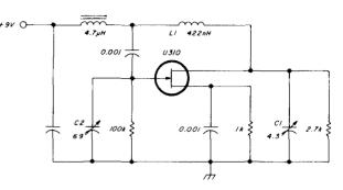
fig. 5. A common-source Colpitts oscillator designed using the procedure described in the text.
