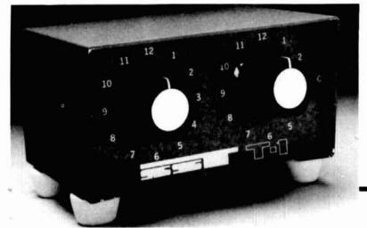
All band operation (160-10 meters) with any random length of wire. 200 watt output power capability-will work with virtually any transceiver. Ideal for portable or home operation. Great for apartments and hotel rooms-simply run a wire inside, out a window, or anyplace available. Efficient toroid inductor for small size: 4-1/4" x 2-3/8" x 3", and negligible loss. Built-in neon tune-up indicator. SO-239 connector. Attractive bronze finished enclosure.
