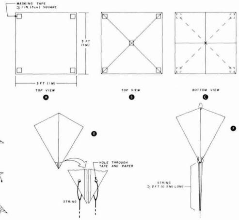
fig. 5. Construction details for the parachute. Sketches A through C show top and bottom views; D through F show assembly details.
