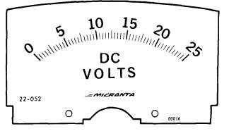
fig. 5. Full-scale meter face after modification.
