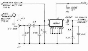
fig. 9. Receiver audio circuit.
