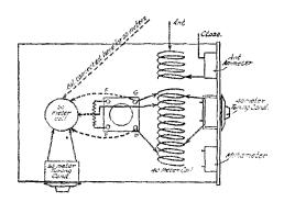
local communication which 40 meters allows, I made up a transmitter which can be shifted from one band to the other and still work efficiently in each band.
