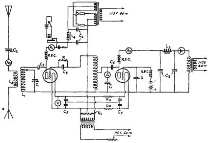
THE CIRCUIT DIAGRAM OF THE TRANSMITTER
