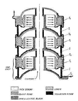
FIG. 6. SKETCH INDICATING INTERNAL STRUCTURE AND CURRENT DISTRIBUTION IN A STACK OF CONDENSERS SUCH AS SHOWN IN FIG. 5
