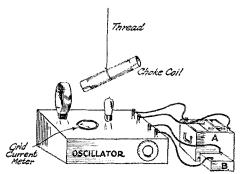
FIG. 1. AN R.F. CHOKE HUNG NEAR AN OSCIL-LATOR WHICH IS PROVIDED WITH A GRID-CURRENT METER CAN EASILY BE INVESTI-GATED FOR RESONANCES. As the tuning dial of the driver is turned the grid meter will indicate the more marked "humps" and
