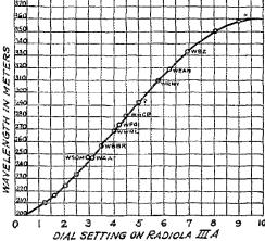
FIG. 2. CURVE MADE FROM BROADCASTING STATIONS IN ABOUT 15 MINUTES
