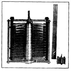
A HIGH-POWER TRANSMITTING CONDENSER COMPARED WITH A MIDGET RECEIVING CONDENSER. THE STEEL SCALE IS ONE FOOT LONG.
