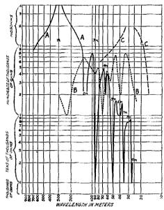
CURVES SHOWING THE MANNER IN THE IMPEDANCE OF R.F. CHOKES WHICH THE VARY WITH FREQUENCY
