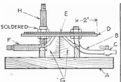
Fig. 1.—A simple yet efficient air-pump. The exhausting platform. A. Baseboard 10 in.  $\times$  10 in.  $\times$  1 in.; B. Bent gas-pipe; C. Gas-tap fitted to B; D. Metal plate 7 in. diameter, about  $\frac{1}{8}$  in. thick; E. Rubber gasket ring,  $6\frac{1}{2}$  in. overall diameter; F. Right-angled Schrader tyre valve without "inside"; G. Platform support, 2 pieces of  $\frac{1}{2}$ -in. wood, each 7 in.  $\times$  2 in.; H. Ordinary short tyre valve with "inside."
