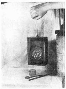
A wooden box containing a 4-lb, weight suspended by a liquid air-cooled piece of frozen metal to its outer
