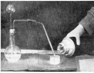
Carbon dioxide gas (CO<sub>2</sub>) is frozen solid as it streams into the glass dish around which liquid air is poured.
