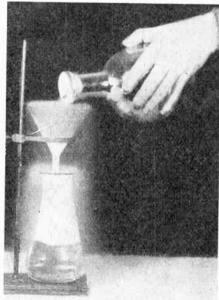
Liquid air being poured from one vessel to another.
