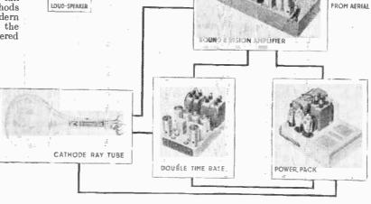
On the left is shown a diagrammatic arrangement of the component assemblies of a G.E.C. television receiver.
