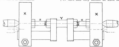
Fig. 3.—The crank ready for chucking.
