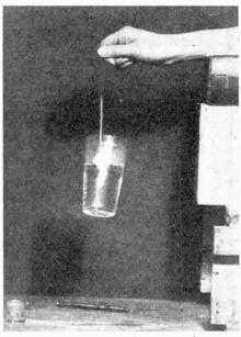
A spectacular experiment. A yale key tied to a piece of string has been cooled in liquid air and then immersed in a tumbler containing hot water. The key has frozen hard to the sides of the glass with the result that the entire tumbler of hot water can be lifted up and held in mid air. Note the coating of frost on the lower half of the string.
