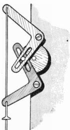
Fig. 4.—A device for giving up- achieving the and-down motion to two rods. same result.
