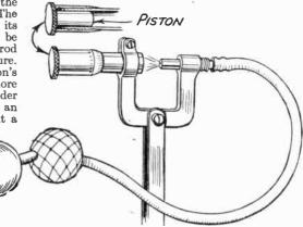
Fig. 3.—Galton's miniature organ pipe in the form of a whistle which was blown by means of a rubber bulb.
