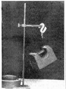
A hook of solid mercury suspending a 7-lb. weight. The mercury has been frozen in liquid air.
