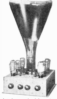
A time-base unit with cathode-ray tube in position, which shows the size of the tube compared with ordinary valves.
