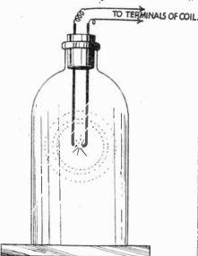
Fig. 5.—Luminous effect of electric spark in partial The spark does not " jump vacuum. as usual, but sets up a luminous glow as pressure decreases.
