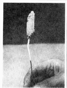
A piece of wire cooled in liquid air and then immersed in a vessel of oil immediately freezes the oil around it into a hard mass. Here is frozen oil on the end of the wire.
