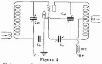
Plate neutralized radio frequency amplifier. This amplifier operates class C whenever the negative bias exceeds cut-off. Note that the coupling links are located close to points of low r.f. potential on the grid and plate tank coils.
