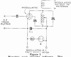
Figure 3 Negative peak clipping indicator. This 0-10 milliammeter in series with the half wave rectifier B (consisting of an 879 in high voltage class C amplifiers) indicates whenever the negative modulation peaks exceed 100%. The rectifier conducts only when the plate of the class C stage goes negative with respect to the filament.
