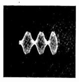
Figure 5 The effect of too little capaci-tance in the final tank con-denser. This causes poor lin-earity and sideband splatter.
