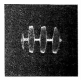
Figure 1 This indicates an overmodulated carrier without carrier shift. The positive peaks cut off at the same point as the negative peaks (100%).
