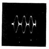
Figure 2 This carrier is also overmodulated but as the positive peaks can swing materially beyond 100% before cutting off carrier shift is produced.
