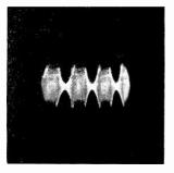
Figure 4 Oscillograph showing bad carrier shift at 80% modulation. High frequency parasitics are also present. This carrier shift was caused by insufficient excitation.
